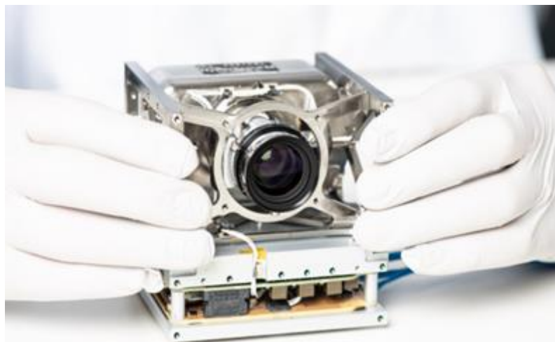
Figure 2 Nanosatellite hyperspectral camera HyperScout® M ( https://satsearch.co )
